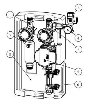
1. BALL VALVE WITH HIGH PARAMETER THERMOMETER
