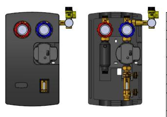
Pump group is a device that ensures and regulates the circulation of the solar fluid between the solar collectors and the tank. The group consists of a circulating pump as well as control and measuring devices. It can be used both for flat solar collectors and for vacuum collectors. The advantage of the double pump group is that it enables controlling the temperature of the solar system heating medium supply and the return.
