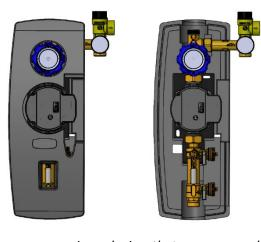
Pump group is a device that ensures and regulates the circulation of the solar fluid between the solar collectors and the tank. The group consists of a circulating pump as well as control and measuring devices. It can be used both for flat solar collectors and for vacuum collectors.
